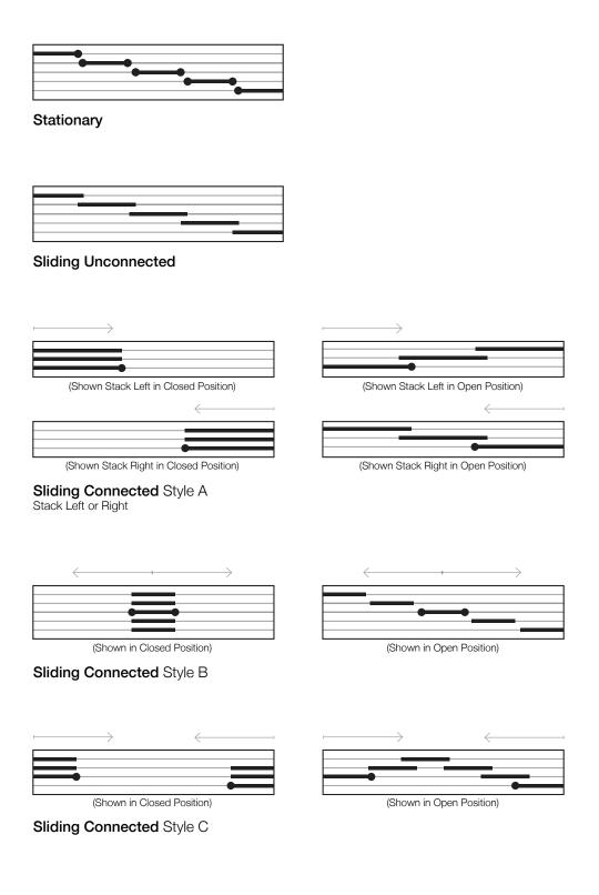
Indicates stopper that secures panel in place—panels without a stopper slide freely
