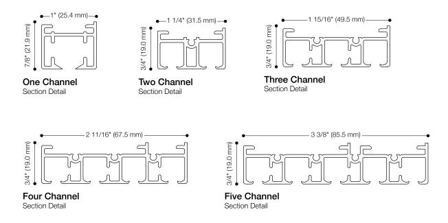
Additional channels may be created by stacking tracks (i.e. six channel track may be created with two three channel sections)
