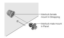
Align male mounts in Panels with female mounts in Strapping and push in until they snap
